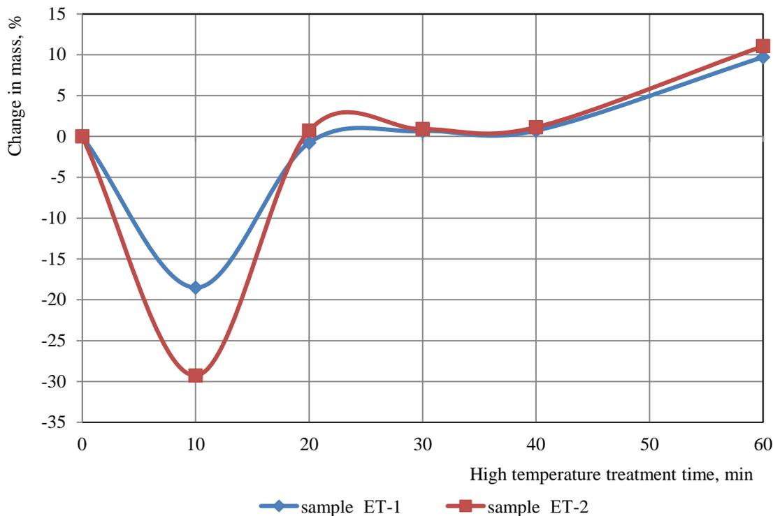
Fig. 2. Change in ore mass during high-temperature processing
