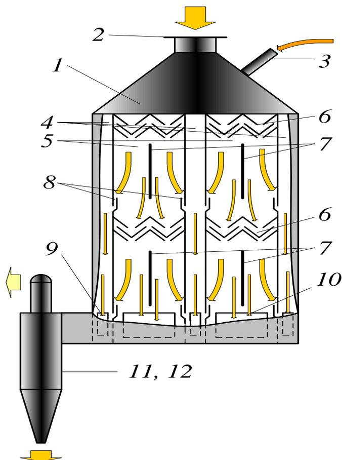
*Fig. 5. Triboelectrostatic separator (diagram): 1 - working chamber; 2 - separation product feed pipe; 3 - additional loading pipe; 4 - negative deflection electrodes; 5 - separator sections; 6 - particle charging devices; 7 - positive deflection electrodes; 8 - horizontal slots; 9, 10 - collectors; 11, 12 - cyclones.*
